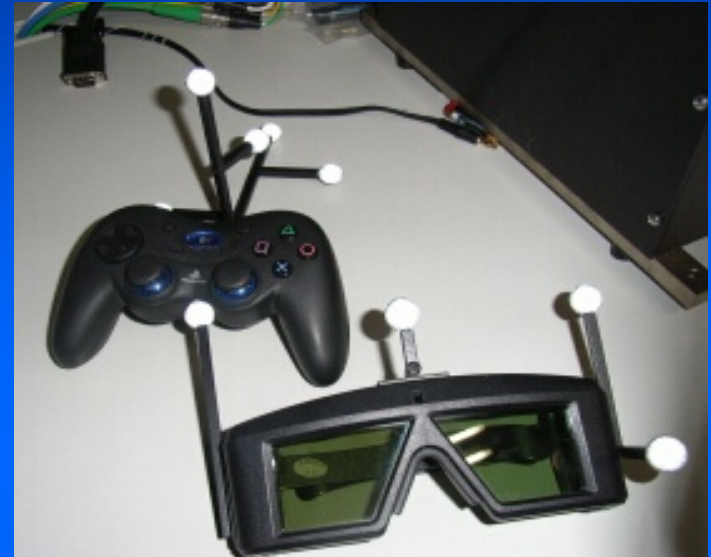
Right: Liquid crystal Shutter glasses Left: Image Controller
